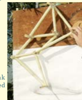
→ This is the link mechanism called "Jansen's link".
