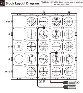
\* Holding onto the lead wire terminals may make it difficult for the circuit to advance to the next stage. If this is the case, touch the terminal of lead wire (A) to (B) (the negative terminal on the circuit board) to discharge the electric charge stored in the 10- $\mu$ F capacitor.
