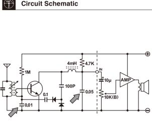
\* Disconnect the antenna if you encounter any beeping dial tone sound at high sensitivity. If you still continue hearing a dial tone even after disconnecting the antenna, swap the 0.05- $\mu$ F and 0.1- $\mu$ F capacitors, making sure to orient them correctly.
