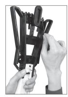
Grip the neck and wind the coil wire around the pickup. Use the hand holding the coil wire to straighten the wire while
