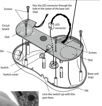
Attach the switch cover to the black switch cap from above at an angle as shown in the picture. If you find it difficult to attach the cover, loosen the screws on the circuit board and move the circuit board back before attaching.
